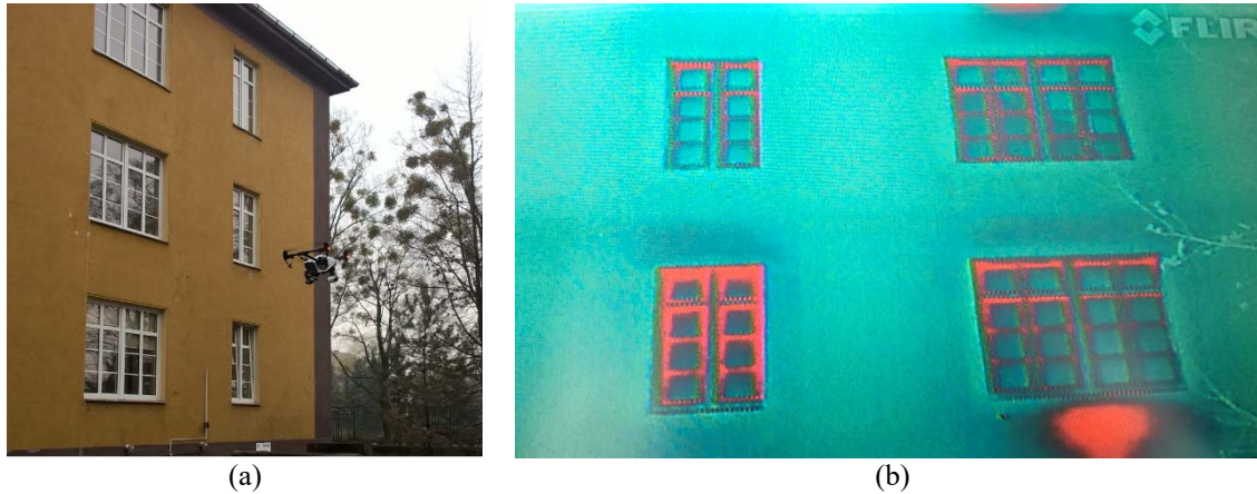
FIGURE 1. Thermal inspection of building with using an UAV. (a) Quadcopter making a thermal inspection of building with using a thermal camera, (b) view from thermal camera
